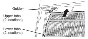
**4.** Replace the air filter to its original position and close the front panel. **Page 23**
