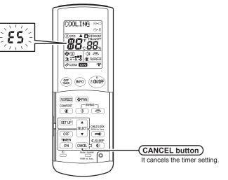
2. The temperature display on the remote controller changes to the error code display and a long beep notifies this indication change.
