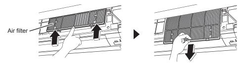
· Push a little upwards the air filter.
