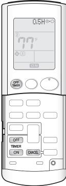
Timer functions are useful for automatically switching the air conditioner on or off at night or in the morning.
