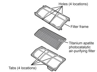
The deodorizing filter for stream and the titanium apatite photocatalytic air-purifying filter do not have front and back sides.
